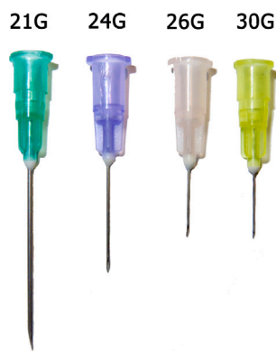
Fig. 13. Medical needles used as nozzles in the proposed weeding machine, with corresponding model names and internal diameters: 21G (0.51 mm), 24G (0.30 mm), 26G (0.24 mm), and 30G (0.15 mm).
