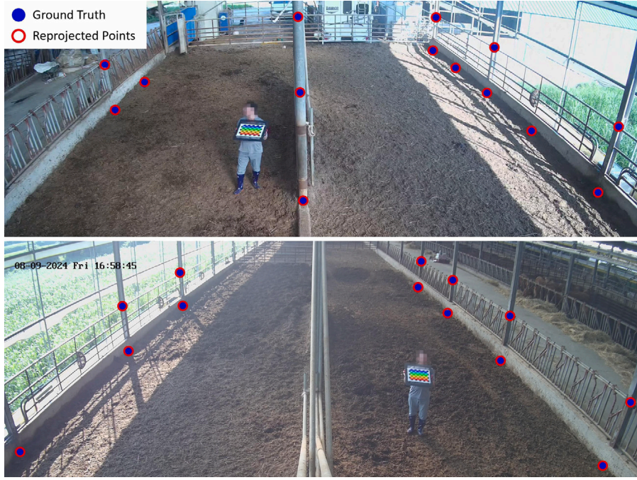
Fig. 4. Camera calibration results from two different viewpoints. Traditional calibration typically relies on detecting keypoints from a printed chessboard or calibration board. However, in this scene, although the board is visible, its distance from the camera limits its coverage and resolution, leading to inaccurate parameter estimation. To address this, we manually selected 2D keypoints as ground truth (blue solid circles) and estimated intrinsic and extrinsic parameters using DLT followed by Levenberg–Marquardt optimization. The reprojected points (red hollow circles) demonstrate the accuracy of the estimated parameters.
