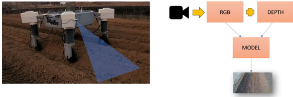
FIGURE 15. (a) The robot setup that shows the view of the real sense camera (b) The real sense camera which can take both RGB and depth images that are combined and given to the model to get the prediction line on the furrow.
